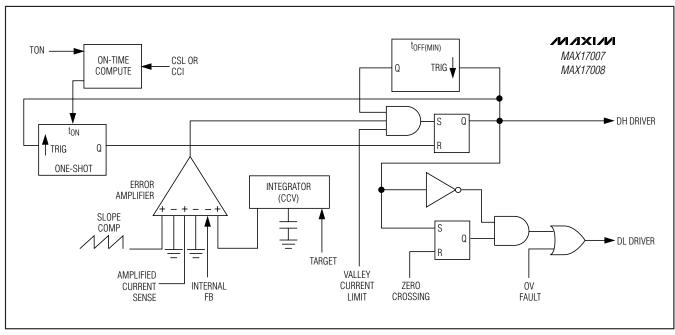
Figure 4. PWM Controller Block Diagram
