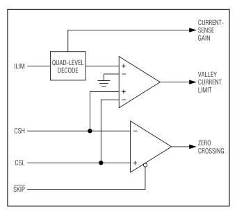
Figure 8. Current-Limit Block Diagram
