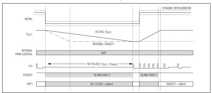
Figure 11. Dynamic REFIN1 Transition (SKIP = GND)
