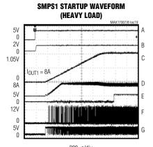
A. EN1, 5V/div E. PG00D1, 10V/div B. REF, 2V/div F. LX1, 10V/div C. V<sub>0UT1</sub>, 500mV/div G. DL1, 10V/div D. I<sub>LX1</sub>, 10A/div
