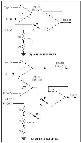
Figure 9. SMPS Target Decode Block Diagram
