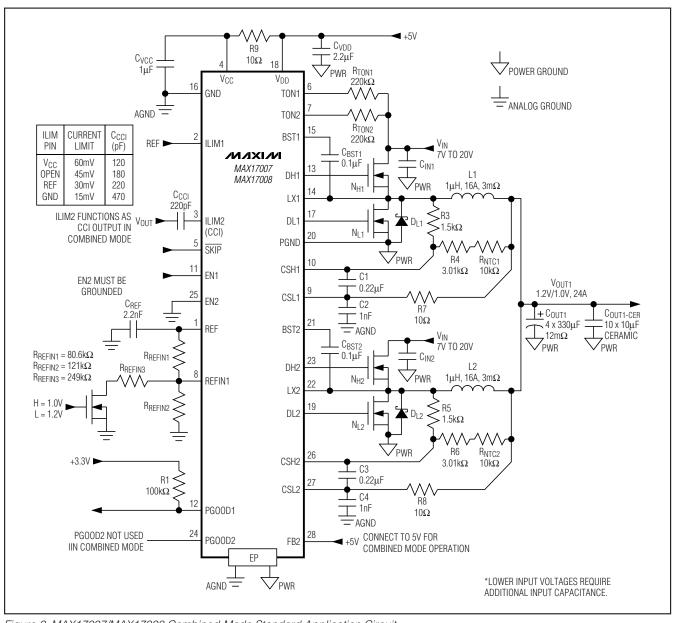
Figure 2. MAX17007/MAX17008 Combined-Mode Standard Application Circuit
