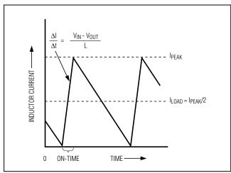
Figure 5. Pulse-Skipping/Discontinuous Crossover Point
