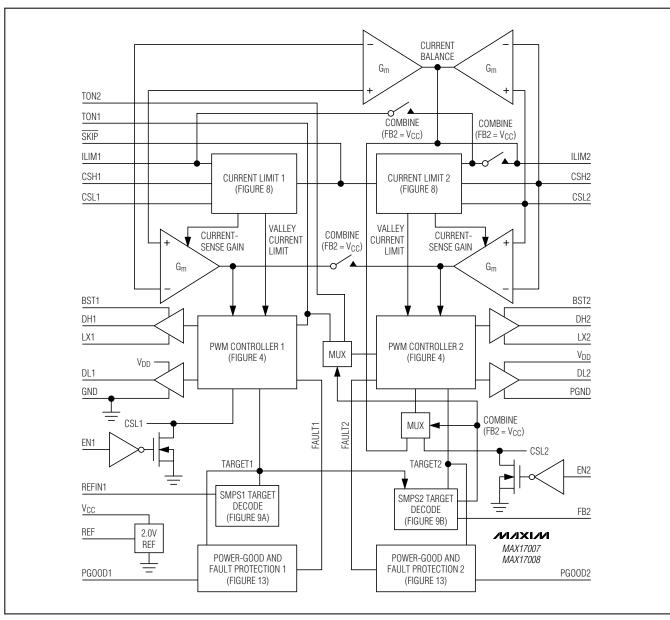
Figure 3. MAX17007/MAX17008 Functional Diagram
