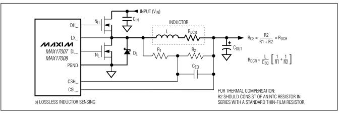
Figure 14. Current-Sense Configurations (Sheet 2 of 2)
