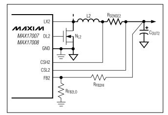
Figure 10. Setting VOUT2 with a Resistive Voltage-Divider
