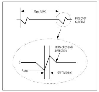
Figure 6. Ultrasonic Waveform
