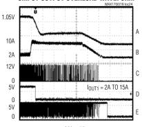
A. V<sub>OUT1</sub>, 500mV/div D. PG00D1, 5V/div B. I<sub>LX1</sub>, 10A/div E. DL1 5V/div C. LX1, 10V/div
