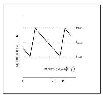
Figure 7. "Valley" Current-Limit Threshold Point
