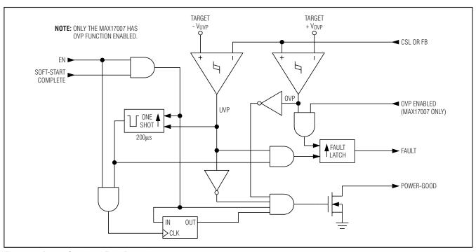
Figure 13. Power-Good and Fault Protection
