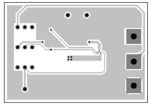
Figure 6. Bottom Layer (Bottom View)
