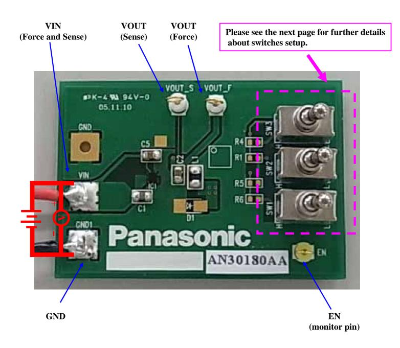
Figure 2. Appearance of Evaluation Board
