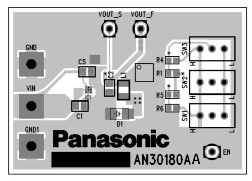
Figure 5. Top Layer with silk screen ( Top View )
