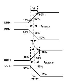
FIGURE 6A. MEASUREMENT POINTS
