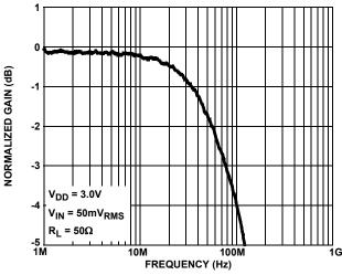
FIGURE 17. FREQUENCY RESPONSE; COM1A AND COM4A
