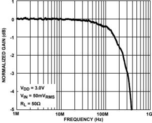
FIGURE 19. FREQUENCY RESPONSE; COM1B and COM4B
