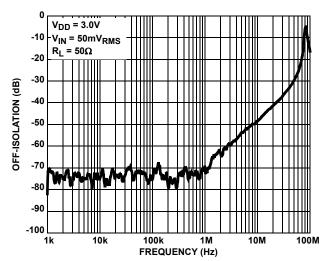
FIGURE 20. OFF-ISOLATION; COM1B and COM4B
