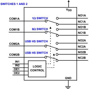
NOTE: Switches shown in Logic "0" position. Logic "0" when INx  $<\!0.5V$
