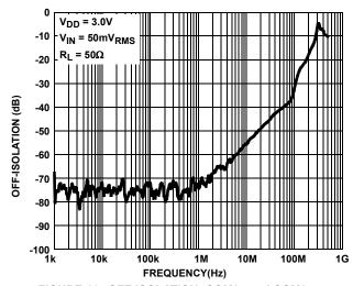
FIGURE 16. OFF-ISOLATION; COM2x and COM3x
