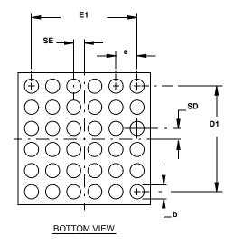
W6x6.36 6x6 ARRAY 36 BALL WAFER LEVEL CHIP SCALE PACKAGE
