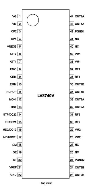
It is short-circuited in IC though there are VM1, VM2, OUT1A, OUT1B, OUT2A, OUT2B, RF1 and RF2 of each of two pins.
