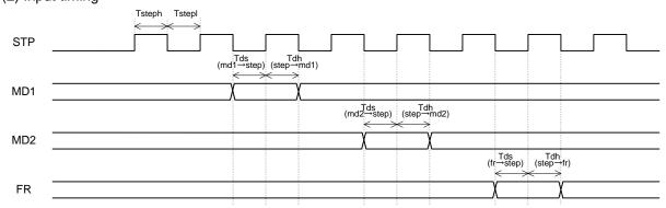
TstepH/TstepL: Clock H/L pulse width (min 500ns)
