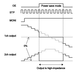
When the OE pin is set High, the output is forced OFF and goes to high impedance. However, the internal logic circuits are operating, so the excitation position proceeds when the STEP signal is input to the STP pin. Therefore, when OE is returned to Low, the output level conforms to the excitation position proceeded by the STEP input.
