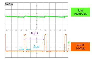
(7) Typical current waveform in each excitation mode when stepping motor parallel input control Full Step (CW mode)
