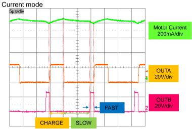
When the motor current reaches to the setting current, it is switched to Slow Decay mode. Motor current switches from Slow Decay mode to Fast Decay mode for 1/16 of one chopping cycle.
