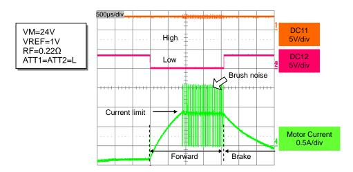
The limit current is set as calculated on the basis of the voltage input to the VREF pin and the resistance between the RF pin and GND using the formula given below.
