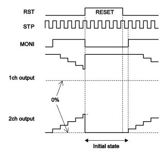
When the RST pin is set to High, the excitation position of the output is forcibly set to the initial state, and the MONI output is placed in the ON state. When RST is then set to Low, the excitation position is advanced by the next STEP input.
