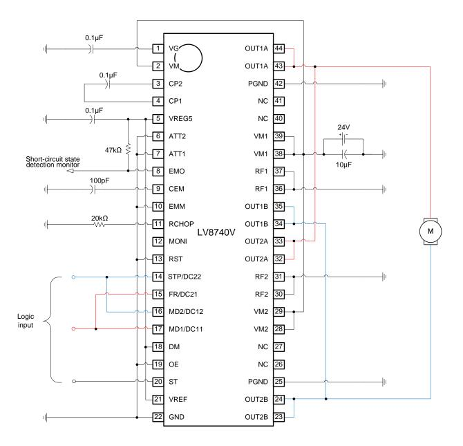
Each constant setting type in the example of the above-mentioned circuit is as follows. Chopping frequency setting.
