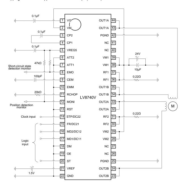
Each constant setting type in the example of the above-mentioned circuit is as follows. When setting current ratio = 100%, VREF = 1.5V, the following output current flows:
