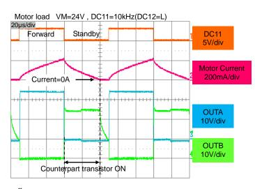
Standby mode turns on the counterpart transistor
