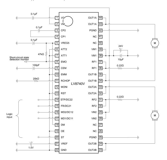
Each constant setting type in the example of the above-mentioned circuit is as follows. When setting current LIMIT = 100%, VREF = 1.5V, the following output current flows :
