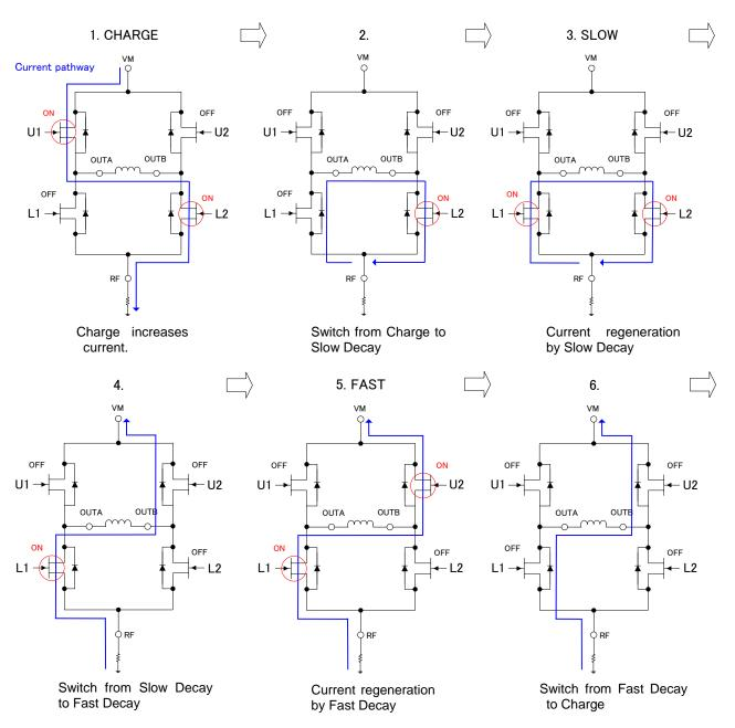
This IC controls constant current by performing chopping to output transistor.
