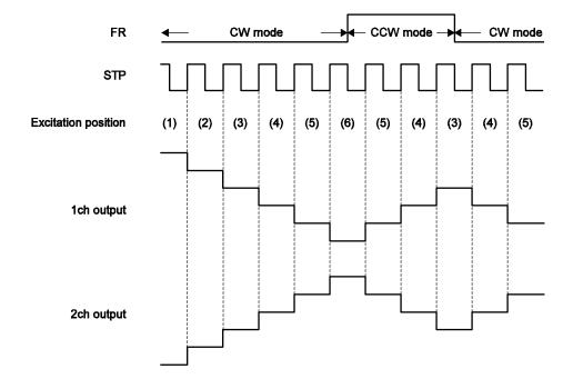
The internal D/A converter proceeds by one bit at the rising edge of the input STEP pulse. In addition, CW and CCW mode are switched by setting the FR pin.
