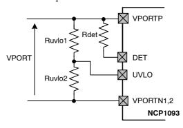
Figure 6. Default Internal UVLO Configuration (NCP1093 only)
