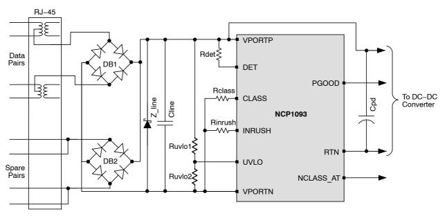
Figure 2. Typical Application Circuit using the NCP1093 with External UVLO Setting
