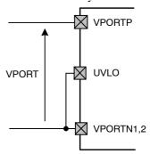
Figure 5. Default Internal UVLO Configuration (NCP1093 only)
