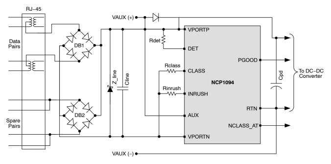
Figure 3. Typical Application Circuit using the NCP1094
