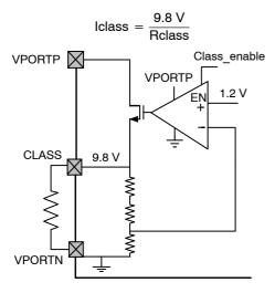
Figure 4. Classification Block Diagram
