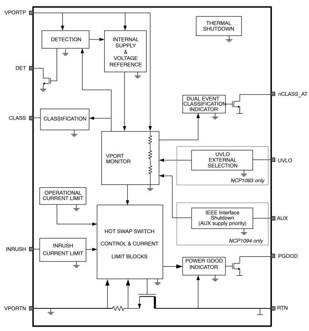
Figure 1. NCP1093/94 Functional Block Diagram
