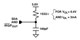
FIGURE 3. STANDARD OUTPUT LOAD FOR TESTING THE DEVICE WITH  $\mbox{\sc V}_{\mbox{\sc DD}} = 5.0\mbox{\sc V}$
