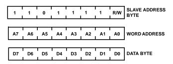
FIGURE 20. SLAVE ADDRESS, WORD ADDRESS, AND DATA BYTES
