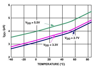
FIGURE 6. I<sub>DD1</sub> vs TEMPERATURE
