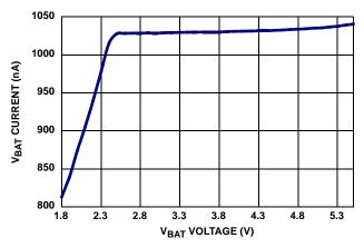
FIGURE 4.  $I_{BAT}$  vs  $V_{BAT}$  ( $V_{DD} = 0V$ )
