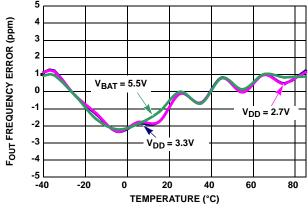
FIGURE 8. OSCILLATOR ERROR vs TEMPERATURE
