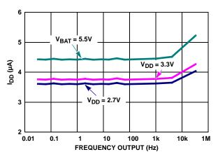
FIGURE 9. F<sub>OUT</sub> vs I<sub>DD</sub>
