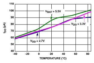
FIGURE 12. I<sub>DD</sub> WITH TSE = 1 vs TEMPERATURE
