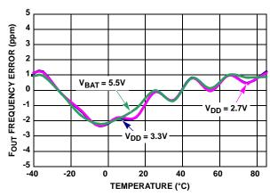
FIGURE 2. OSCILLATOR ERROR vs TEMPERATURE
