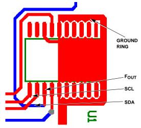
FIGURE 23. SUGGESTED LAYOUT FOR THE ISL12022M
