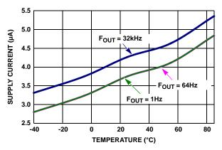
FIGURE 10. I<sub>DD</sub> vs TEMPERATURE, 3 DIFFERENT F<sub>OUT</sub>
