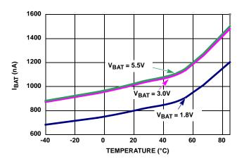
FIGURE 5. I<sub>BAT</sub> vs TEMPERATURE (V<sub>DD</sub> = 0V)
