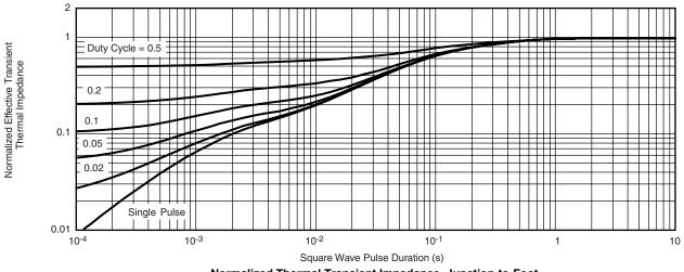
Normalized Thermal Transient Impedance, Junction-to-Foot
