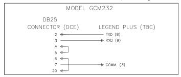
For connection to an RS232 port on a computer, refer to diagrams below.
