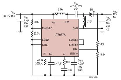
C<sub>IN</sub>, C<sub>DC</sub>: MURATA GRM21BR61E475KA12L C<sub>OUT</sub>: MURATA GRM32ER61C226KE20 D1: VISHAY SILICONIX 30BQ040 L1A, L1B: COILTRONICS DRQ127-100
