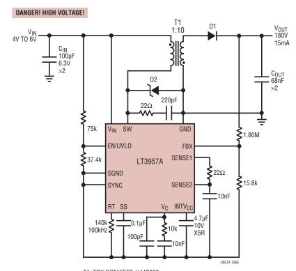
T1: TDK DCT15EFD-U44S003 C<sub>IN</sub>: GRM31CR60J107ME39L
