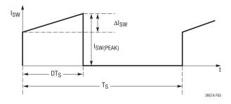
Figure 3. The Switch Current During a Switching Cycle
