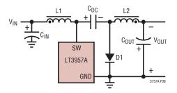
Figure 8. A Simplified Inverting Converter
