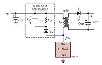
Figure 6. A Simplified Flyback Converter
