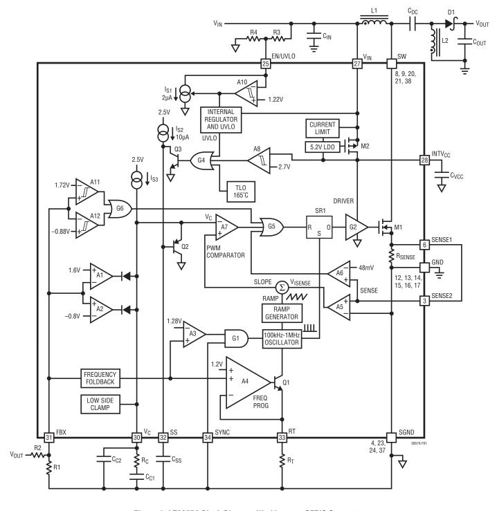
Figure 1. LT3957A Block Diagram Working as a SEPIC Converter
