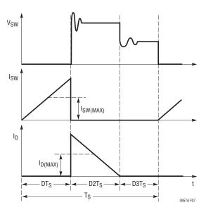
Figure 7. Waveforms of the Flyback Converter in Discontinuous Mode Operation
