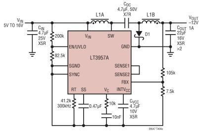
C<sub>IN</sub>: MURATA GRM21BR61E475KA12L C<sub>DC</sub>: TAIYO YUDEN UMK316BJ475KL C<sub>OUT</sub>: MURATA GRM32ER61C226KE20 D1: VISHAY SILICONIX 30BQ040 L1A, L1B: COILTRONICS DR0127-100
