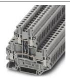
Component terminal block, for installing components that can be individually selected, Connection method: Screw connection, Cross section: 0.14 mm² - 6 mm², AWG: 26 - 10, Width: 6.2 mm, Color: gray, Mounting type: NS 35/7,5, NS 35/15
