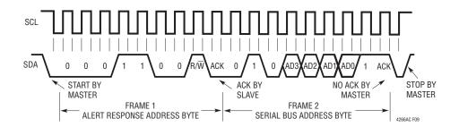
Figure 9. Reading from Alert Response Address
