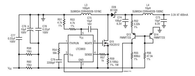
Figure 15. Positive V<sub>DD</sub> Boost Converter
