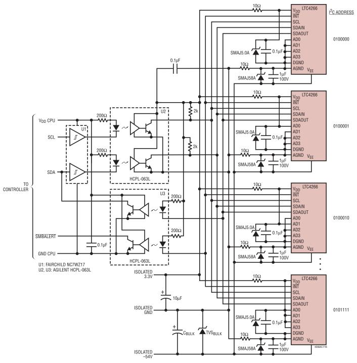
Figure 16. Opto-Isolating the I<sup>2</sup>C Bus
