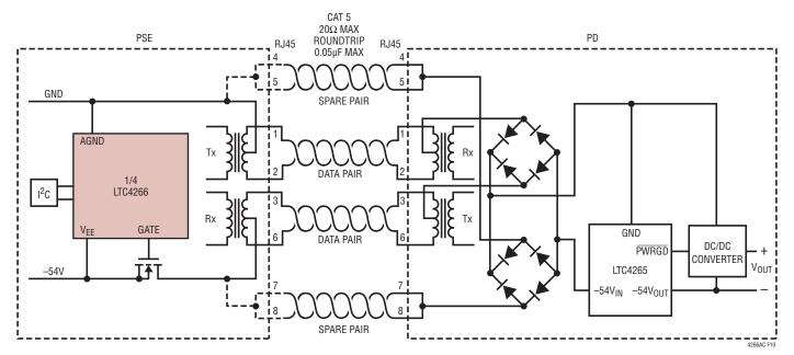
Figure 10. Power Over Ethernet System Diagram
