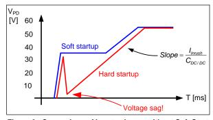
Figure 3. Comparison of input voltages without Soft Start (Hard startup), and with Soft Start (Soft startup).
