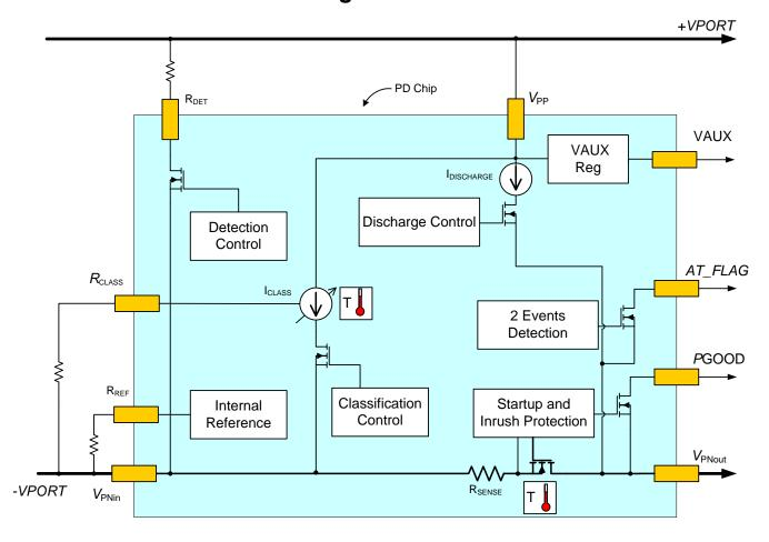
Figure 2: PD70200 Functional Block Diagram
